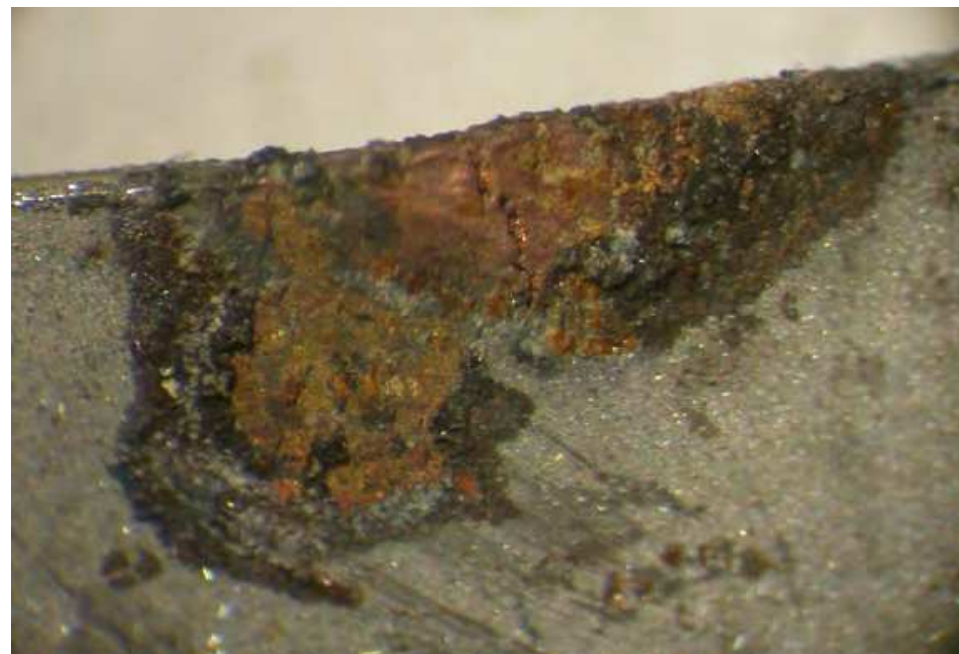
Figure 10: Deposits on the surface of the copper alloy clip in contact with nail A2 (magnification 40x)
