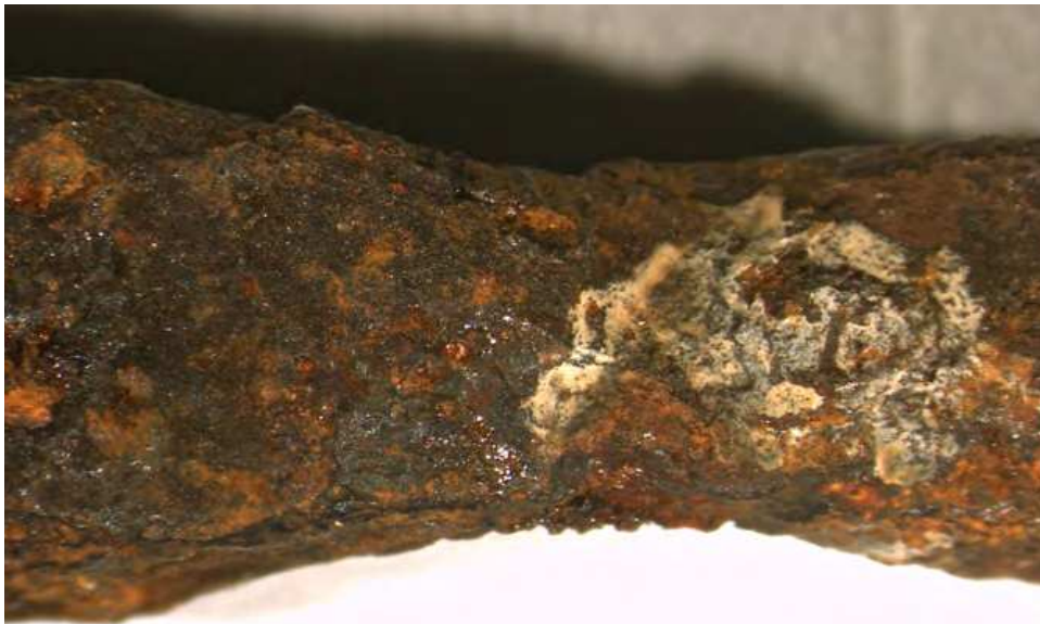
Figure 6: View of nail A1 showing loss of material and white adherent, approximately 20 mm from point (magnification 6x)
